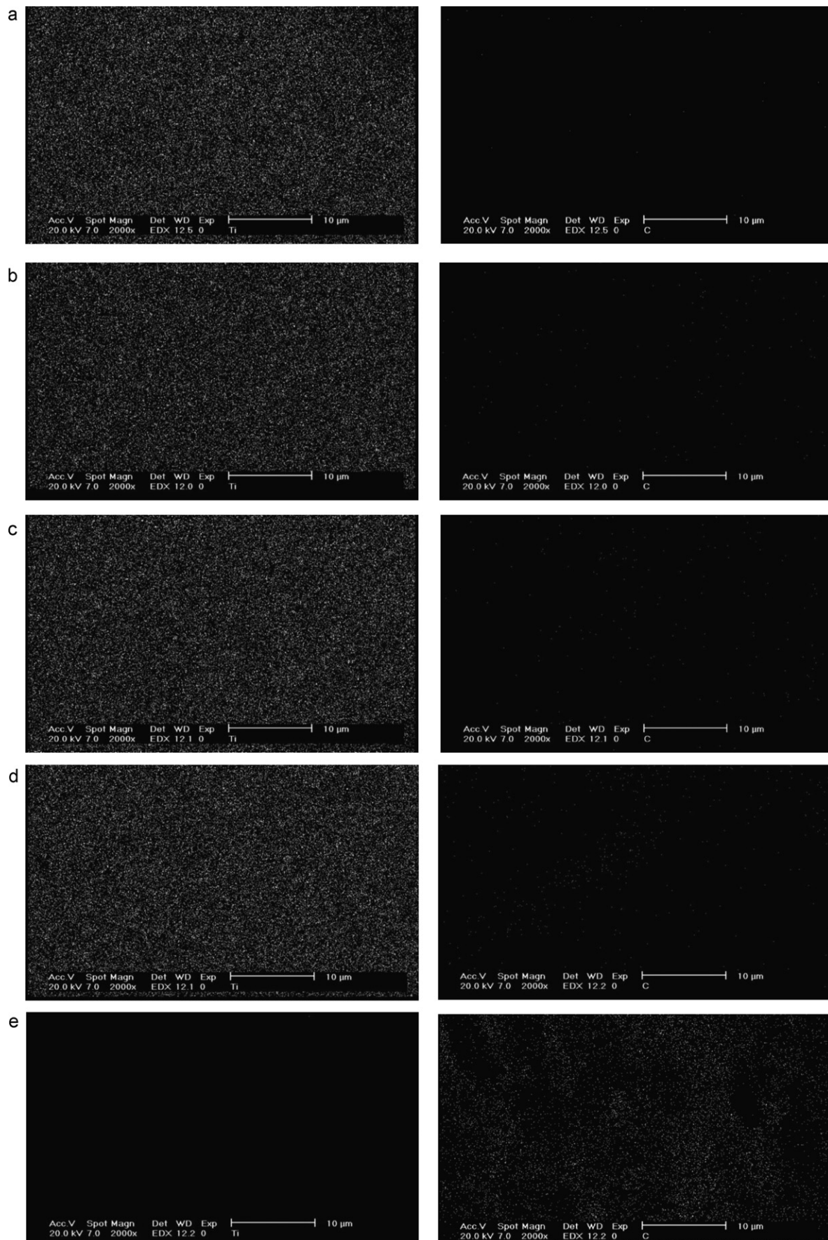
Fig. 4. WDX of immobilized composite photocatalyst (titania nanoparticle–Canola hull activated carbon) at different wt.% of Canola hull activated carbon: (a) 0, (b) 1, (c) 2, (d) and 3 (e) pure Canola hull activated carbon.
